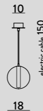
1573.18.1L SOSPENSIONE / HANGING LAMP Glass Ø18 cm - cable 150 cm G9 1 x max 33W 230V IP20
