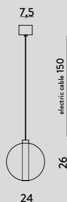
GIG1293.1L SOSPENSIONE / HANGING LAMP Glass Ø24 cm - cavo/cable 150 cm G9 1 x max 42W 230V CE IP20 1m
