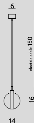
1293.1L SOSPENSIONE / HANGING LAMP Glass Ø14 cm - cavo/cable 150 cm G9 1 x max 42W 230V CE IP20 1m
